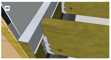
Layer the housewrap over the ledger flashing, and the siding over the housewrap [4A]. Install the joists, but don't mash them against the ledger and compress the flashing—let them breathe [4B]. Treat the joist ends to reduce water absorption.
