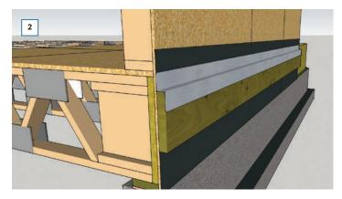
Install Z-style ledger flashing with a hemmed drip edge that extends over the face of the ledger and pushes water away from it.
