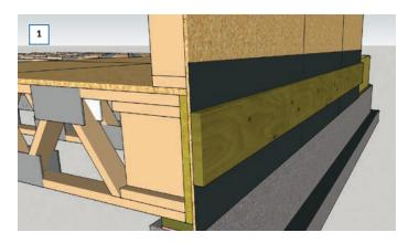
Apply peel-and-stick membrane over the base of the wall where the deck ledger will be. This will protect the sheathing from water and will help to seal fastener holes, too. Install the deck ledger—spaced off sheathing or not—with the appropriate fasteners (through-bolts are better than lag screws; nails and deck screws are unacceptable).
