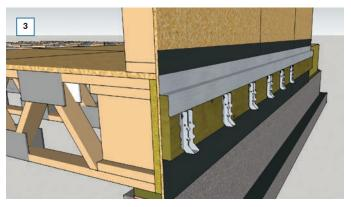
Select joist hangers one size down from the joist depth (such as 2x6 hangers for 2x8 joists) so that they fit below the ledger flashing. Consult a joist hanger sizing chart for exact choices.
